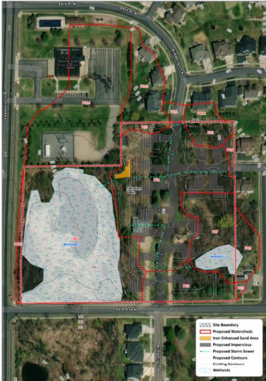
Figure 3 Proposed Drainage Plan
